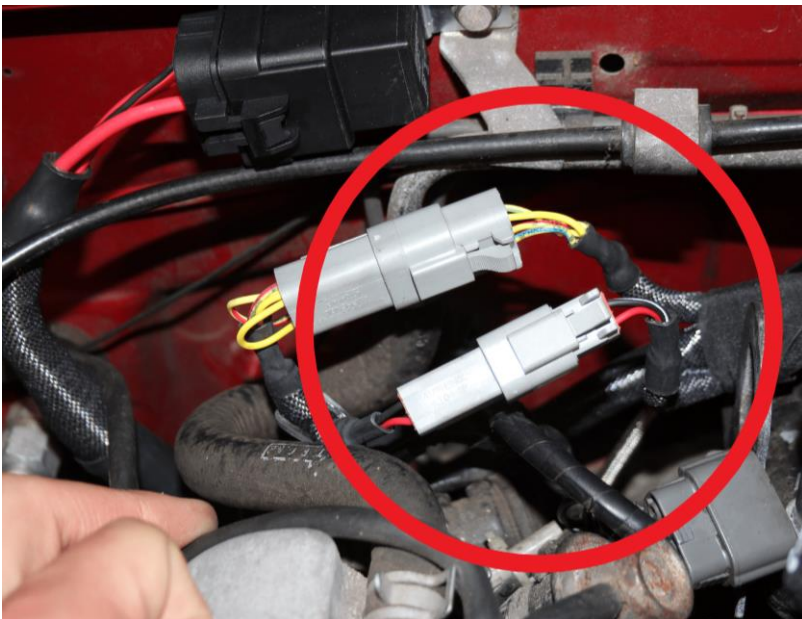
(Figure 14) Primary to Secondary Harness Connection
